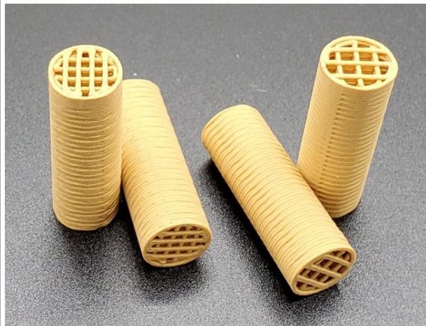
Cordierite ceramic monoliths with high resolution (200 – 400 cps) Lattice designs have excellent thermal shock resistance.
