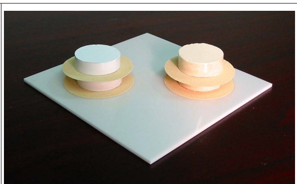
Figure 3b. Medium sized ceramic discs stacked with heavier-grade SPS Sheets inserted between each disc prior to firing
