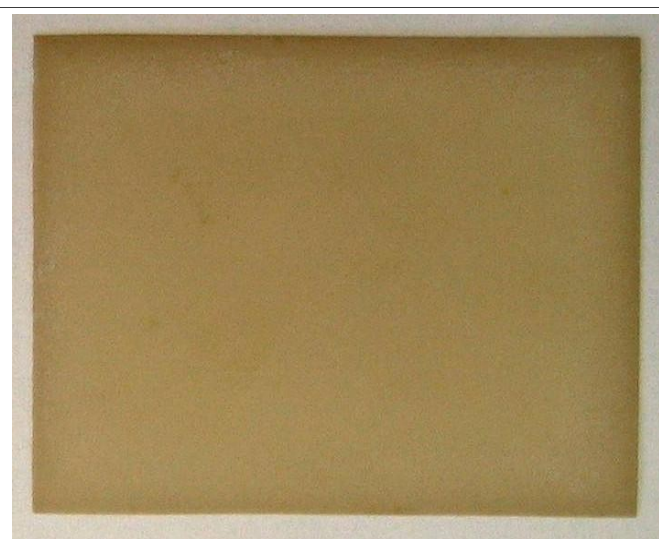
Figure 4b. An identical PLZT plate that was fired using fine grade zirconia SPS Sheets is flat, crack-free, and exhibits high surface quality.
