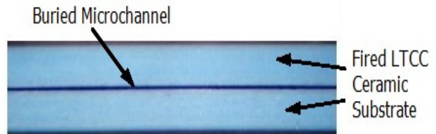
Figure 5. Cross section showing buried microchannels formed in LTCC laminates with thermally fugitive C12 Carbon paste (approx. 40um).
